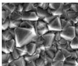
High hardness diamond coating (Hv 10,000) provides excellent wear resistance
